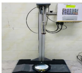
Figure 9. Falling Dart Impact Test
