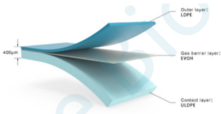
Figure 3. Structure of LeKrius® Film
